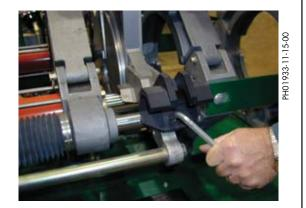
Support the facer with a person or sling so it does not fall once the facer locking bolts are removed.
