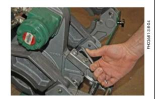
Lift facer out of the carriage and set on cardboard or wood blocks off of ground.
