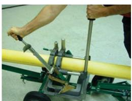
This table is only valid when using a torque wrench and adapter used as shown in the picture above. A 1/2" drive 100 ft-lb 15.0" torque wrench with the torque wrench adapter. Using a torque wrench of a different length will result in different forces from the torque reading.
